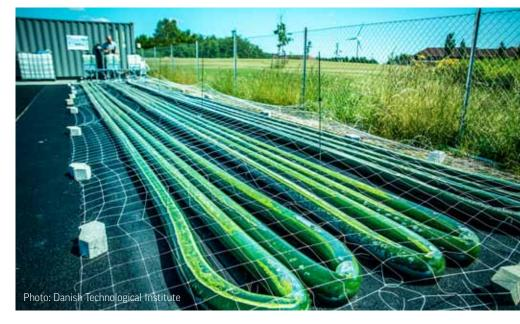
The ambition is to produce microalgae with CO<sub>2</sub> and nutrients from the side streams of biogas production
