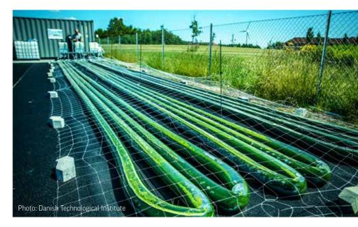
The ambition is to produce microalgae with  $\mathrm{CO}_2$  and nutrients from the side streams of biogas production
